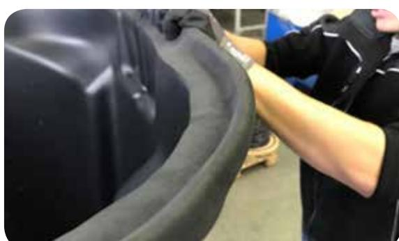
Adhere the seal firmly into position
