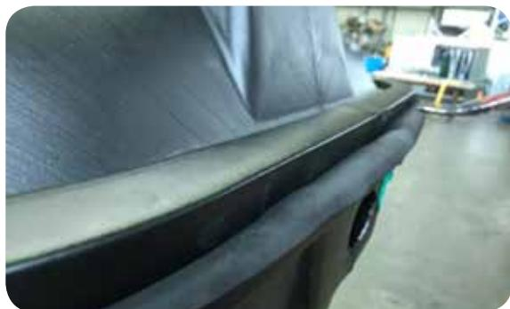
Slot into position, taking care of the seal
