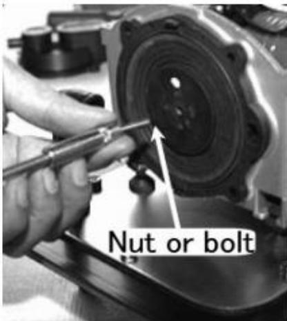
i) Undo the nut or bolt and remove the diaphragm (Nut: SLL series & EL-60, 80-15 & 120W. Bolt: EL-80-17, 100, 150 & 200).
