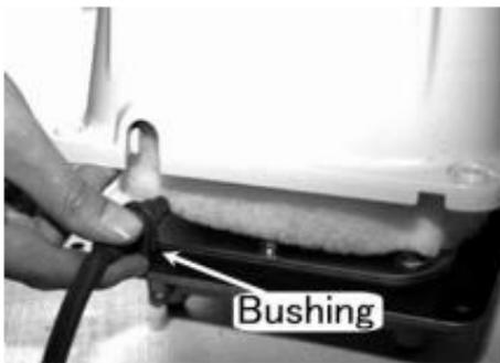
u) Insert the power cord bushing into the location notch.
